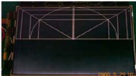
Horizontal Block Gate TAB IC Defect
